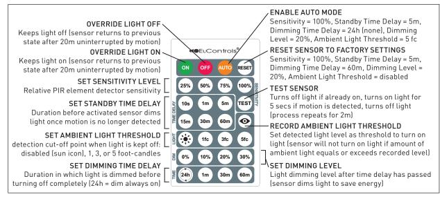
To enable the Force-Off Function which keeps lights off in high traffic outdoor applications, enter these remote commands:
